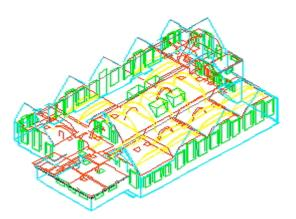
With the observation and recording of both internal and external detail an accurate 3D Computer Aided Design (CAD) model can be produced.
